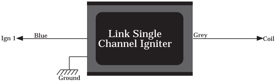
Figure 3.8 (a). Distributor setup with conventional igniter signal (Ign).
